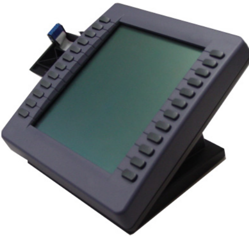
Figure 8: The IP Phone KEM
