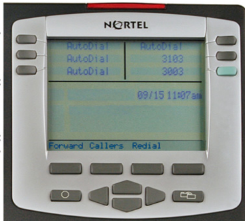
Figure 2: IP Phone 2004 LCD display areas
